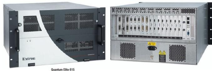
**Extron Quantum Elite Video Wall Processor**
